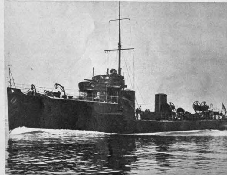
RAISED FORECASTLE appeared with H.M.S. Waveney of 1904 "E" or "River" Class. Earlier turtleback forecastle boats had lower silhouette, but this improvement gave destroyer distinctive outline.
